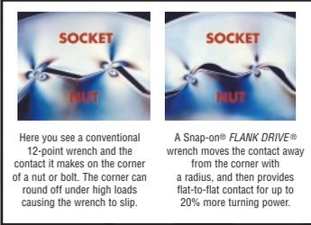
Here you see a conventional 12-point wrench and the contact it makes on the corner of a nut or bolt. The corner can round off under high loads causing the wrench to slip.
